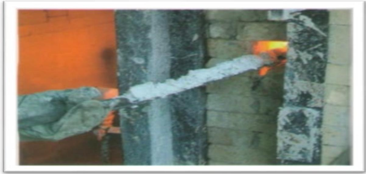
3. As for the third method, it is by spraying sodium carbonate and colored oxides in the oven after mixing it with water, and as it is known that sodium carbonate is characterized by its solubility in water, and is not dissolved in acids, as in Figure (4) (Branfman, 2009, p50)
