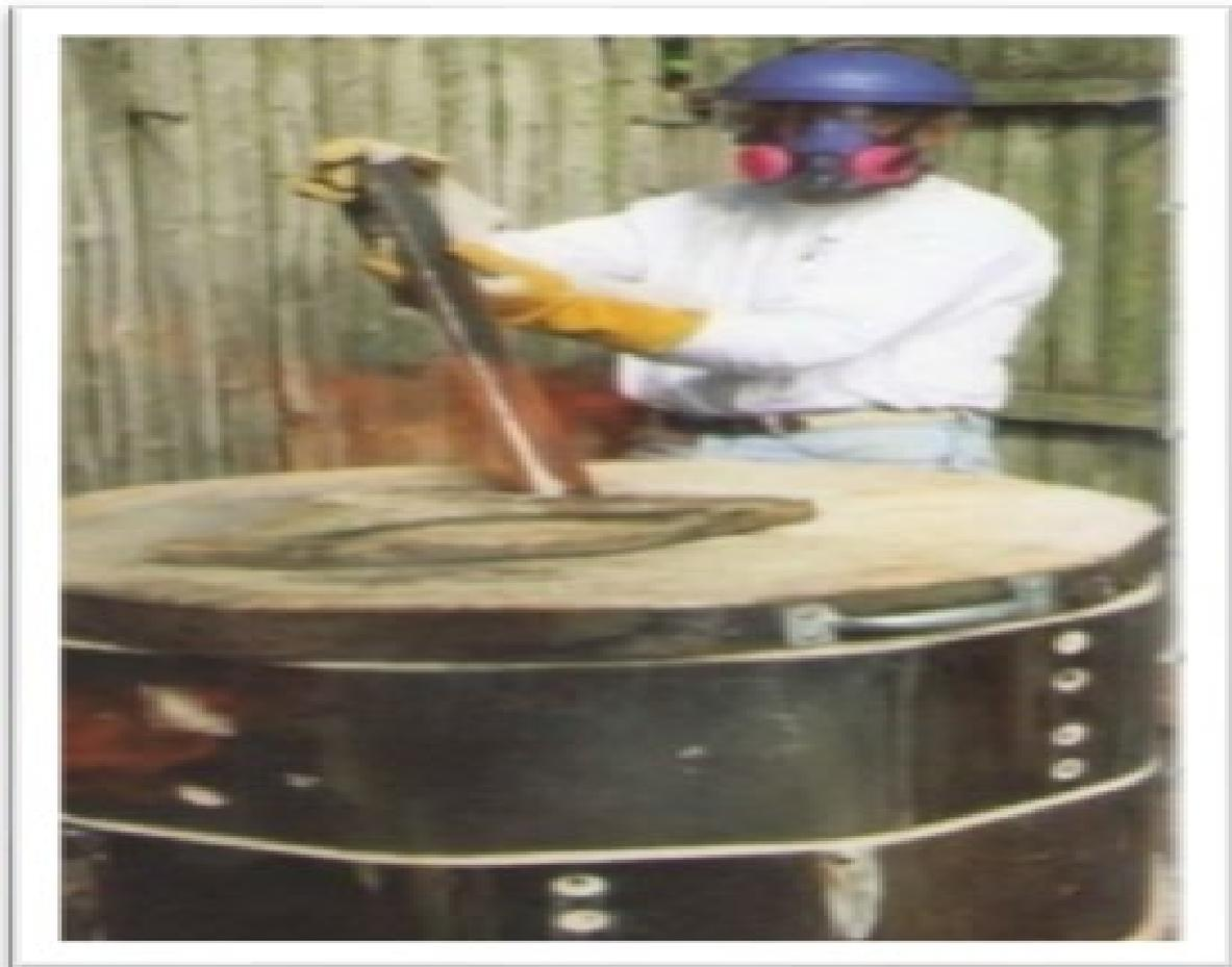
2. Sodium carbonate is inserted with colored oxides in the form of a paste through the combustion opening, after mixing it with water to facilitate the evaporation process, as well as mixing with sodium bicarbonate and calcium carbonate. As in Figure (2-3) (Nichols, 2006, p. 8).
