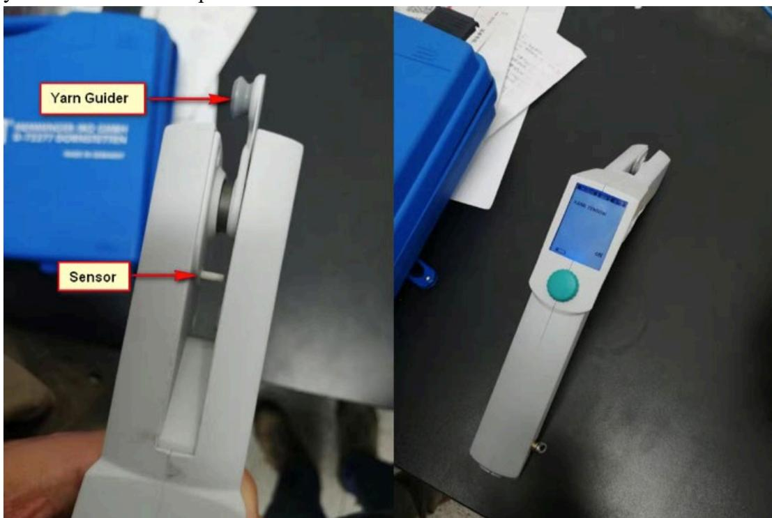
**Figure 1.** Digital tensioner device
