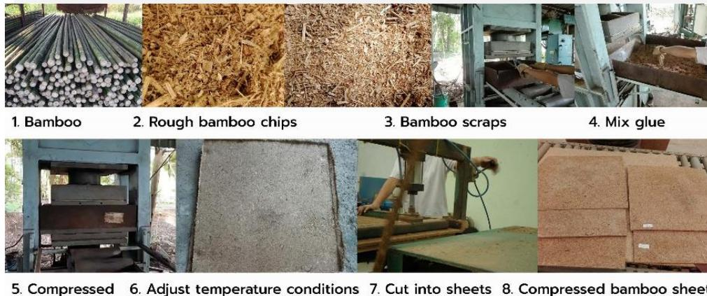
Figure 4. The process of making wood framing sheet for weaving into a Lam Pan mat
