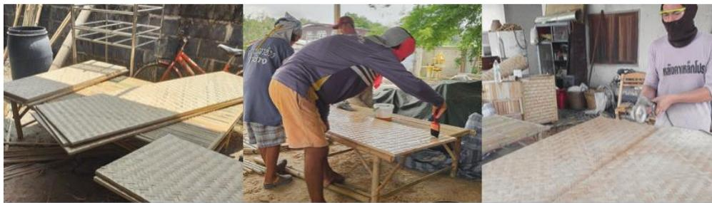
Figure 5. covering the mat and applying glaze
