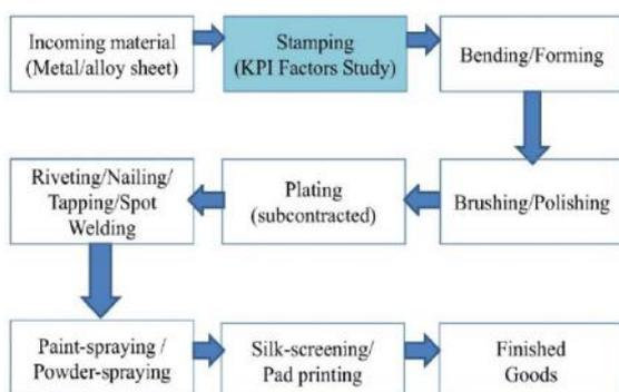
**Figure 2.** Metal Manufacturing Processes Photos
