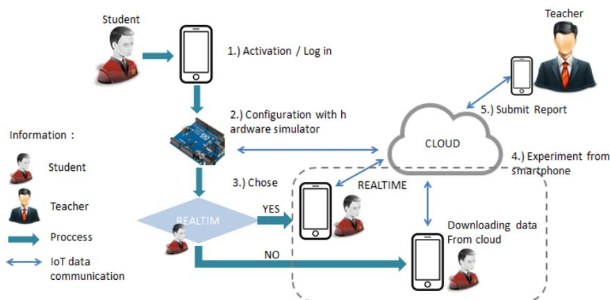
Figure 6. Functional Diagram
